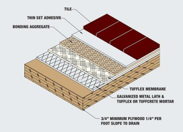
TUFFLEX Anti-Fracture System:
